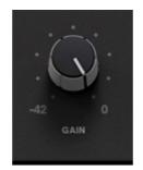
Turn the **GAIN** knob in the input section to control the level of the incoming audio signal. The post-gain signal level is shown above.
